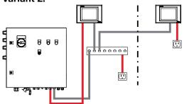
Suction module with two display panels and the necessary switch with power supply 120 V (220 V). One display panel set up at the suction module or in the vicinity of the control unit. Power supply (24V) from the control unit. A further display panel, e.g. in a monitoring room, with individual power supply 120 V (220 V) to supply power.
