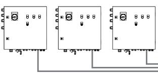
Several suction units with two display panels and a switch with power supply 120 V (220 V). One display panel set up at the suction module or in the vicinity of the control unit. Power supply (24V) from the control unit. A further display panel, e.g. in a monitoring room, with individual power supply 120 V (220 V) to supply power.
