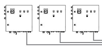
Several suction units with one display panel and a switch with power supply 120 V (220 V). Display panel set up at the suction module or in the vicinity of the control unit. Power supply (24V) from the control unit.
