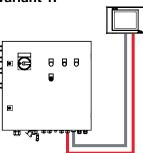
Suction module with control unit and **one** display panel either on the suction module or in the vicinity of the control unit. Power supply (24 V) for the display panel from the control unit.
