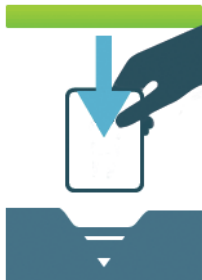
Fig. 7: Example of the animation prompting for insertion of the phosphor storage plate
