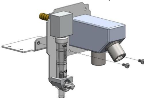
4. Attach assembled GCS to chair adapter bracket using remaining 2x M4 screws. **\*Orientation of bracket varying depending on chair, consult your chair bracket's instructions for further information\***. Attach the breathing/scavenger circuit and breathing bag to the front of the GCS, check for leaks, and the system is ready for use.
