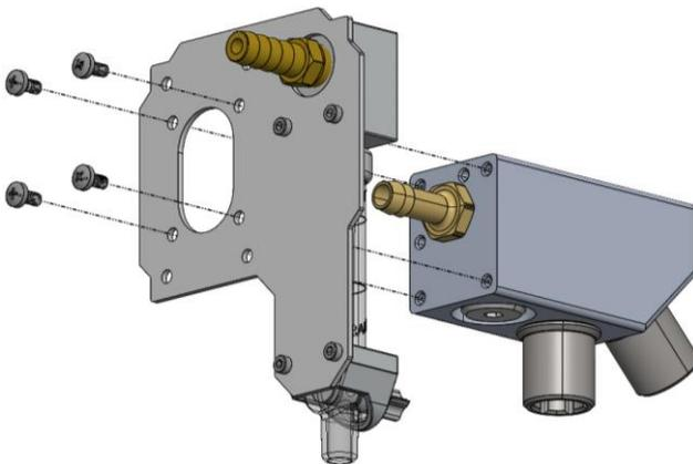
2. Prepare the GCS. Attach the bag tee to the GCS plate using 4x M4 screws. Locate the mixed gas barb on the bag tee and press on the mixed gas hose fed from the unit. Lastly, locate the 3/8" vacuum barb and affix the vacuum tubing. Connect the other end to an available vacuum outlet. **\*Cut tubes to desired lengths and use barbed adapters for junction box applications if needed\***. **\*Hose connections may be made after hardware installation if application requires\***.
