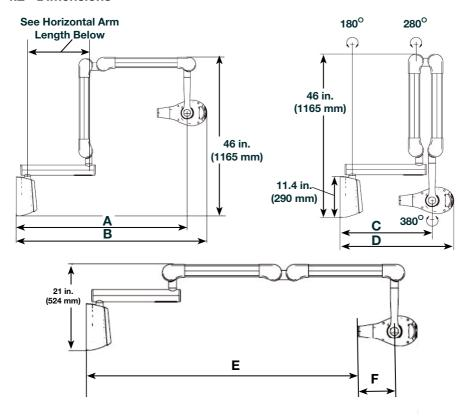
DIMENTIONS 'A' THRU 'E' : SINGLE POST WALL MOUNTING PLATE (P/N A6389) - ADD 0.5" (13mm) 16 CENTER TO CENTER WALL MOUNTING PLATE (P/N A6341) - ADD 1.0" (26mm)
