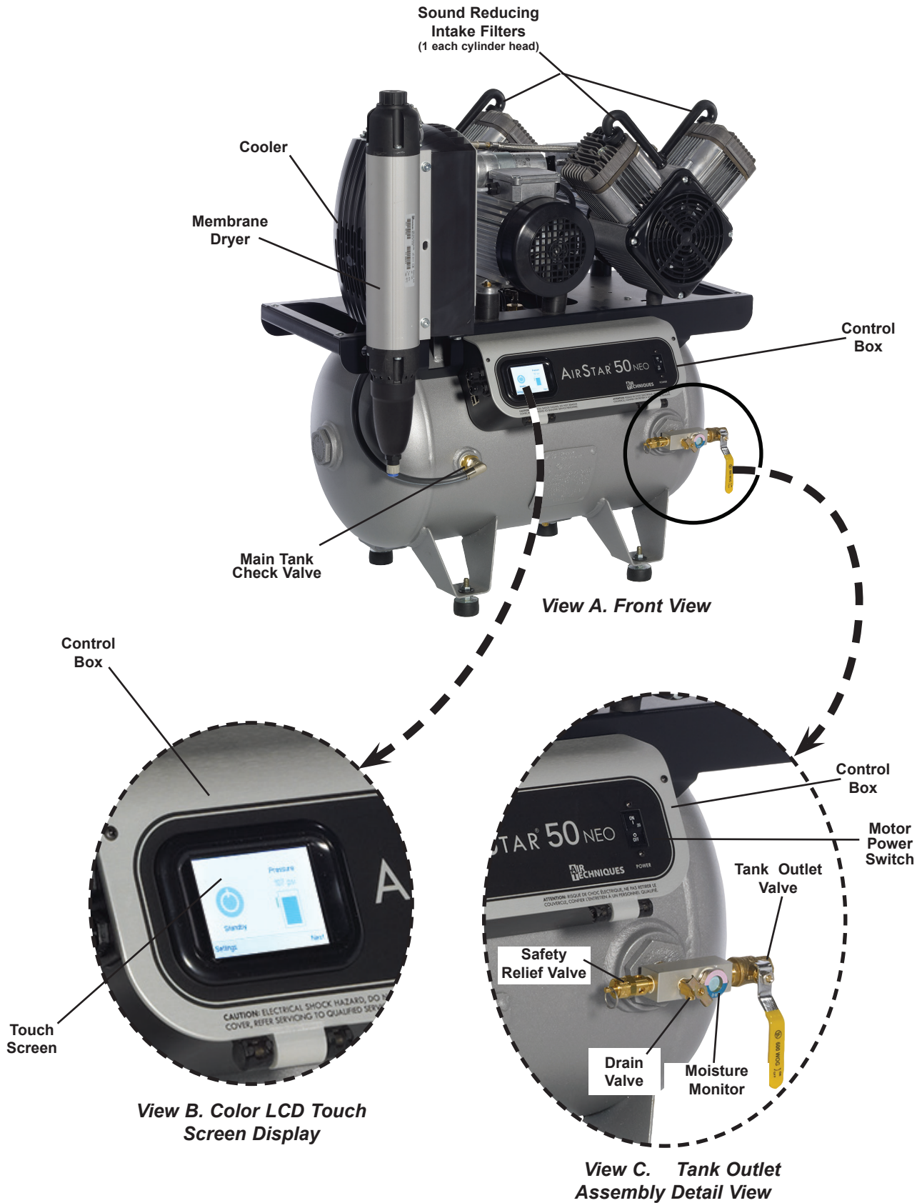
Figure 1. AirStar NEO Parts Location
